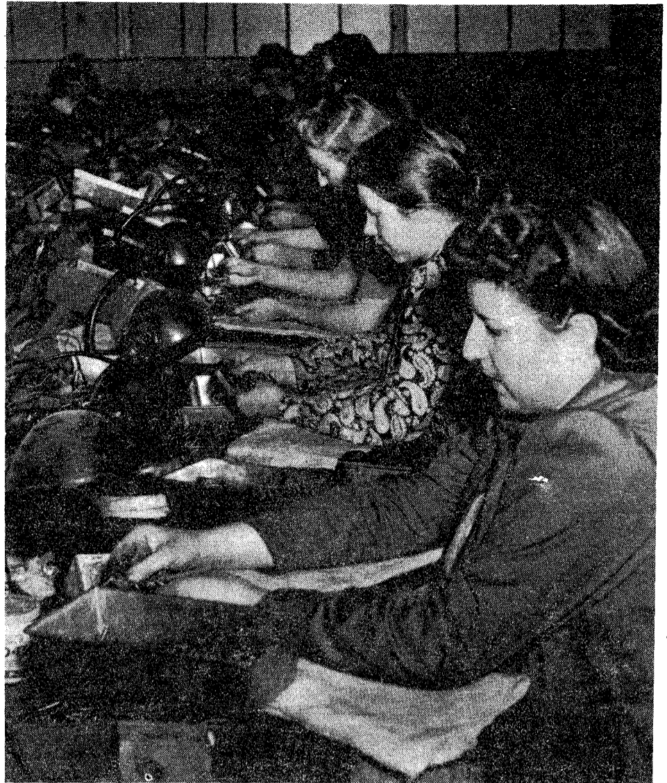
World War II armament production at Animal Trap Company (now Woodstream Corp.) The trays are being filled with bullets. (Photo courtesy of Woodstream Corp.)
