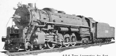
4-8-4 Type Locomotive for Fast Freight Service Built for the Wabash Railway Cylinders 27 in. x 32 in. Drivers, diam Weight, total engine 454,090 lb.
