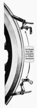
A slight vent of air exhausting with the oil, through the oil shoes, as they are held firmly against the flanges, serves to overcome the centrifugal force at high speed, and assures positive application of the oil.
