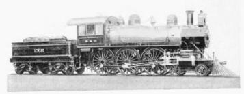
Ten-Wheeled (4-6-0) Type Locomotive for Passenger Service Built for the Baltimore & Ohio Railroad, 1896 Cylinders 21 in. x 26 in. Drivers, diam. 78 in. Weight, total engine 145,000 lb.
