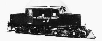
One of the two 70-ton Baldwin-Westinghouse Battery locomotives used by the Twin Branch Railroad for switching service. Exide-Ironclad Batteries supply the power.
