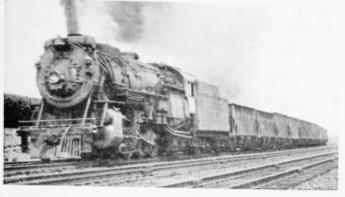
A heavy Mikado recently built by Baldwin. Tender equipped with DAVIS Solid Truss Brake Beams.
