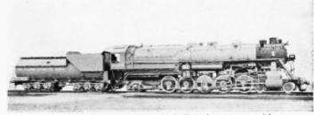
Baldwin Three-Cylinder 4-10-2 Type Locomotive with Water-Tube Firebox. 1926
