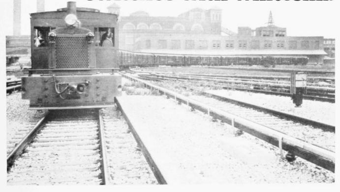
With equal efficiency and with decided economy, a standard 30-ton mechanical drive Whitcomb Locomotive, runs about the yards at the 207th Street Terminal, busily switching and transferring passenger cars for the New York Board of Transportation. In use for some time it is giving "perfect satisfaction," an example of the unfailing, service-free performance of all Whitcombs.
