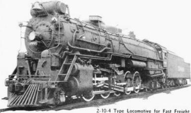
2-10-4 Type Locomotive for Fast Freight Service on Heavy Grade Divisions Built for the Santa Fe System Cylinders 30 in. x 34 in. Drivers, diam. 69 Weight, total engine 502,260 lb.
