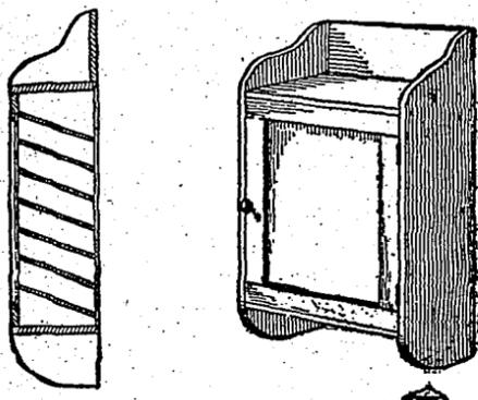
In the design for a closet for holding pot covers herewith illustrated the sides of the cover closet are cut as shown and shelves are nailed between them at a slight angle. No dimensions are given, as the space and the sizes of the covers are not always the same. The back is covered with thin boards placed vertically. The front can be covered with a curtain or a paneled door, as shown.—Popular Mechanics.
