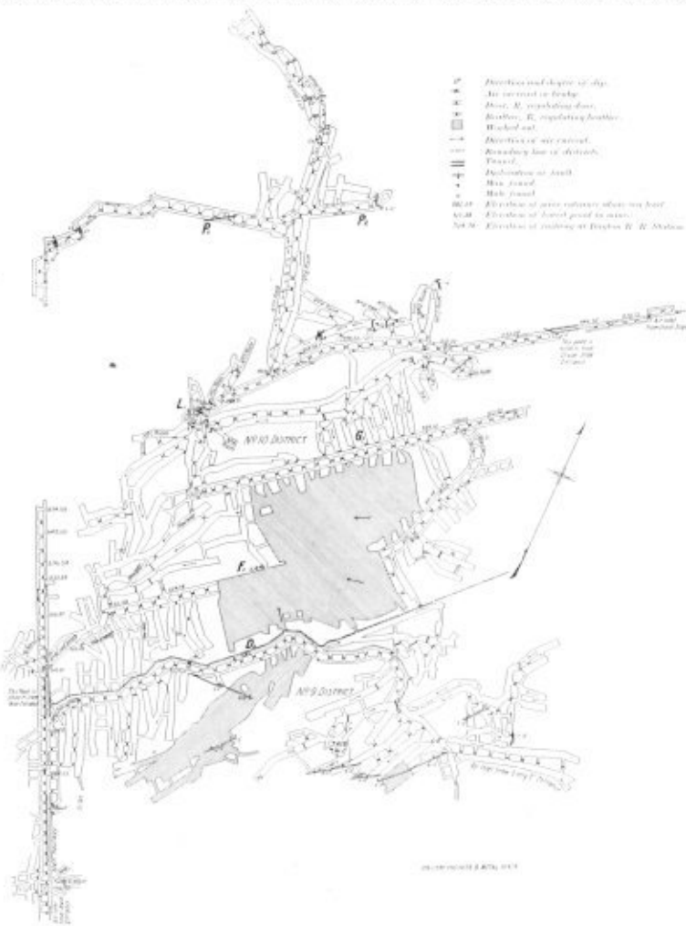
PLAN OF DISTRICTS NOS. 9 AND 10, NELSON MINES, DIXON, TENN. SCALE, EAS. = 100 FT.
