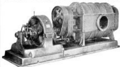
ROOT BLOWER, WITH SLOW SPEED ELECTRIC MOTOR (GENERAL ELECTRIC CO.)
