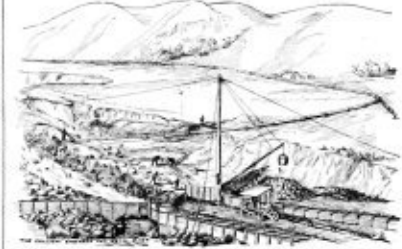
FIG. 6.—"GROUND SLUICING" AND CLEANING BED ROCK.
