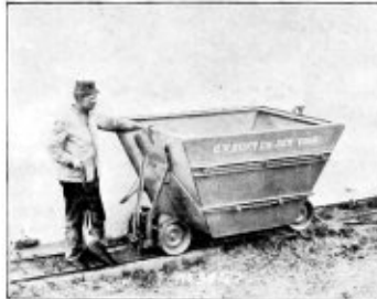
FIG. 4.—COKE CAR BUILT FOR THE TORONTO GAS COMPANY, TORONTO, CANADA.
