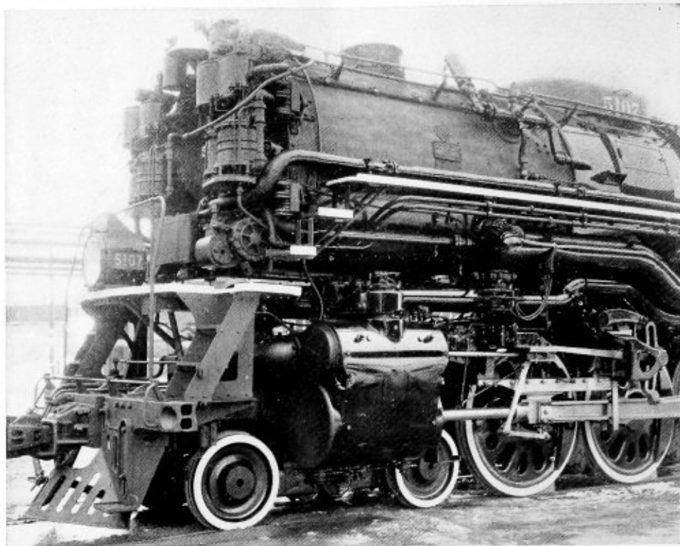
Front end of Northern Pacific 4-6-6-4 type locomotive
