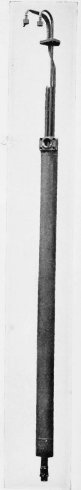
Fig. 4.—Superheater element partially withdrawn from evaporator tube
