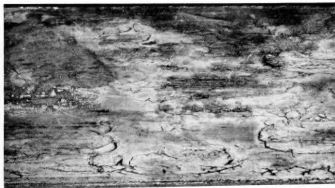
"Eight inch defective Sheet Bar showing how the surface has been burned."
