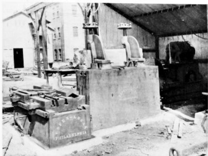
"Showing Cold Saw used for splitting ingots."
