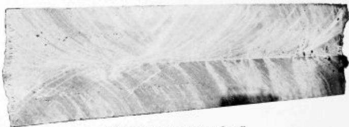
"Split Ingot, typical Armco Iron."
